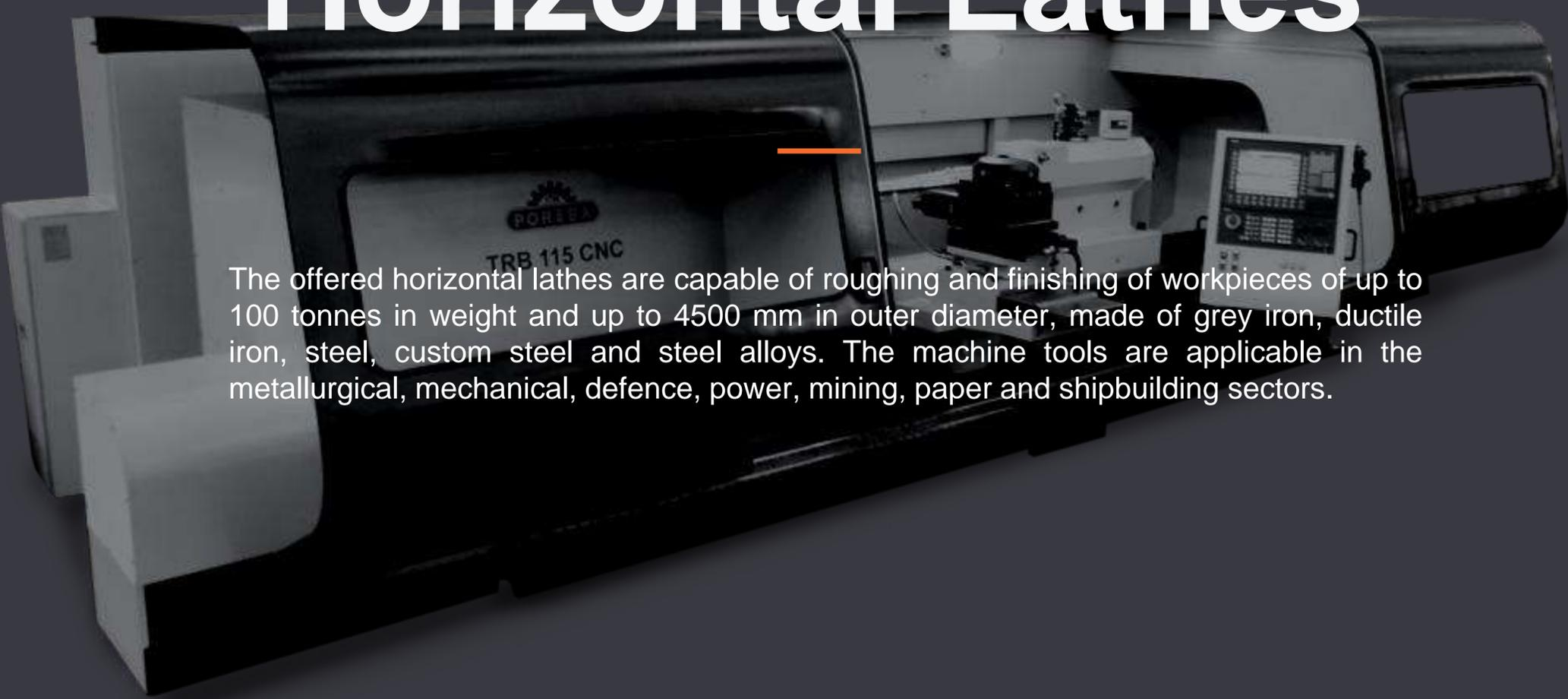
The offered horizontal lathes are capable of roughing and finishing of workpieces of up to 100 tonnes in weight and up to 4500 mm in outer diameter, made of grey iron, ductile iron, steel, custom steel and steel alloys. The machine tools are applicable in the metallurgical, mechanical, defence, power, mining, paper and shipbuilding sectors.
