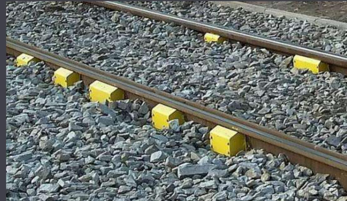
**The wheel profile flat spot detection system** operates on the base of vibrations recorded by a series of vibroacoustic sensors installed in track while a vehicle is running on the length of approximately 10 meters.\*
