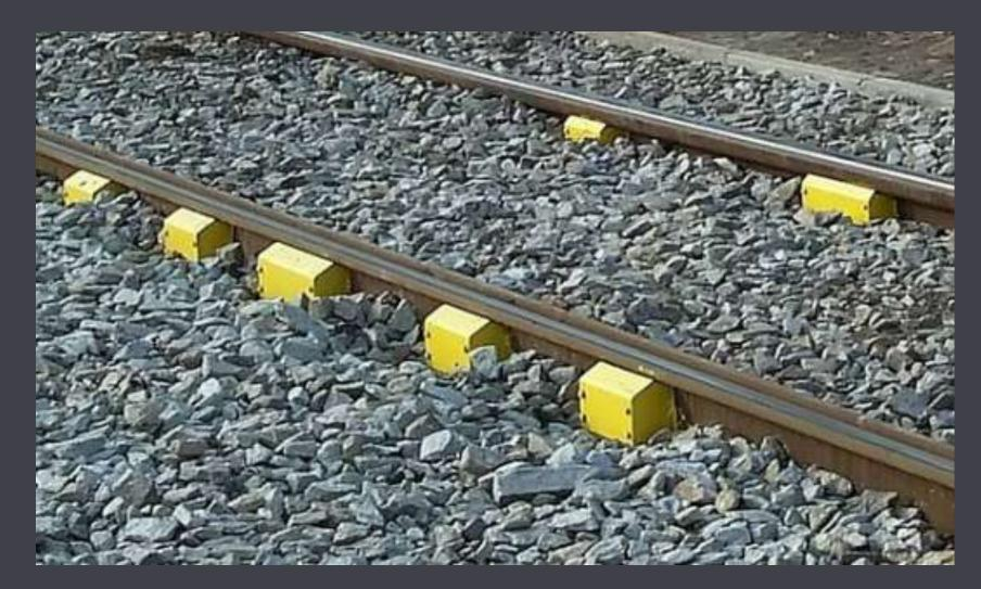
The laser measuring system for wheelsets is designed for monitoring of wheel profile wear. The degree of wheel profile wear is determined on the base of a virtual picture of wheel surface created from the measured data.\*
